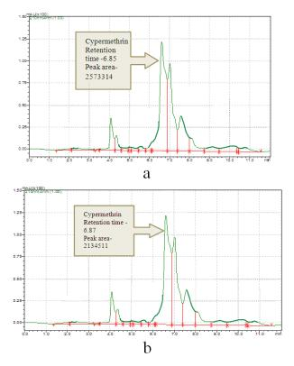
Figure 2. a) Chromatogram of the standard cypermethrin, b) Chromatogram of cypermethrin pesticide residue in tomato samples
