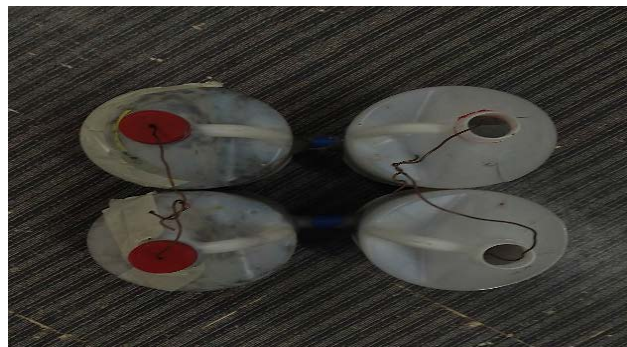
Figure 1. Actual Structure of the Series Microbial Fuel Cell
