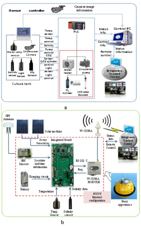
Figure 5. (a) DLAP: The scope and extent of technology for a standard model for development, configuration and backup (b) ELAP: Sustainable energy harvesting, floating technology, wireless technology, and control-room management system.
