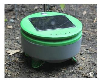
Figure 4. Solar lawn weeder for slashing weeds in lawn [4]
